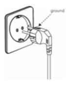
This unit is equipped with the grounded plug. Use a grounded outlet for safe operation.
